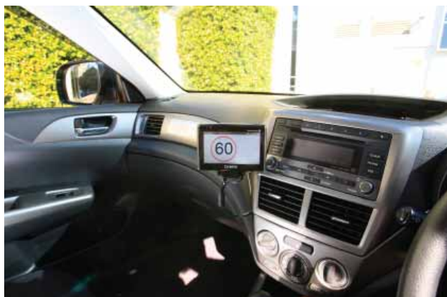
The ISA technology on trial warns drivers when they travel over the speed limit.
