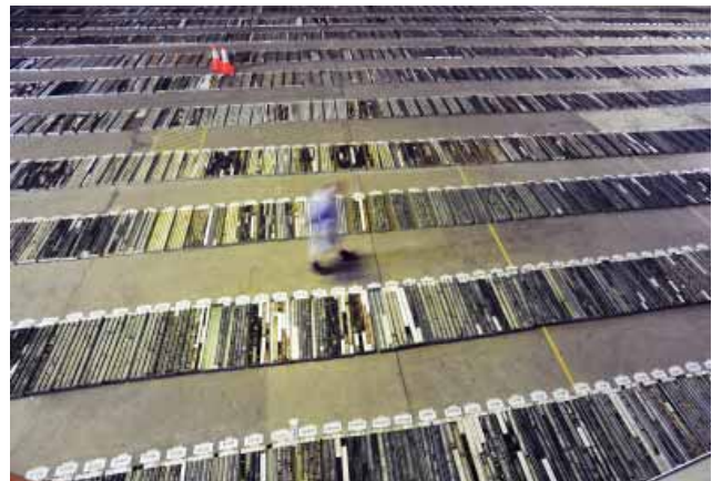
Hundreds of core samples were extracted from the ground for analysis as part of geotech investigations for the Hunter Expressway project.
